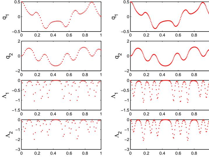
FIG. 4.1. Double pendulum in descriptor form: left  $H = 1/80s$ , right  $H = 1/160s$ . The subplots show the time-evolution of the angle  $q_1$  between the first pendulum rod and the vertical, the angle  $q_2$  between both rods, and the Lagrange multipliers  $\Lambda_1, \Lambda_2$
