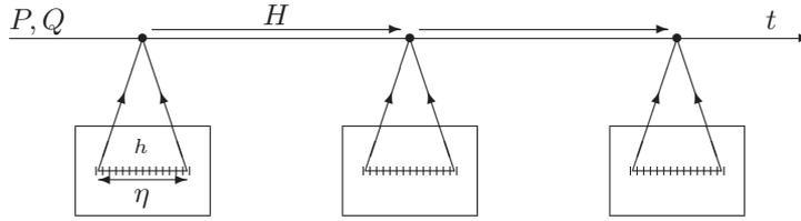
FIG. 2.3. Schematic description of the relation between macro and micro integration: asynchronous algorithm
