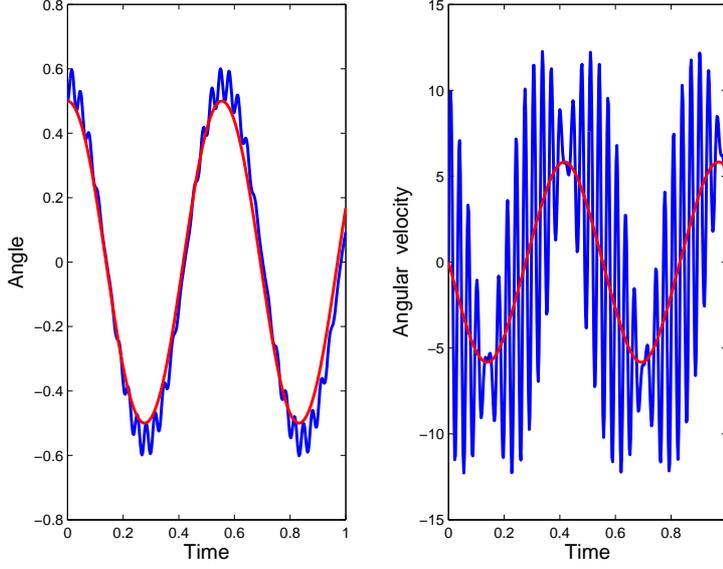
FIG. 2.1. Behavior of pendulum angle  $q$  and angular velocity  $\dot{q}$  for vibratory angular frequency  $\omega = 200$
