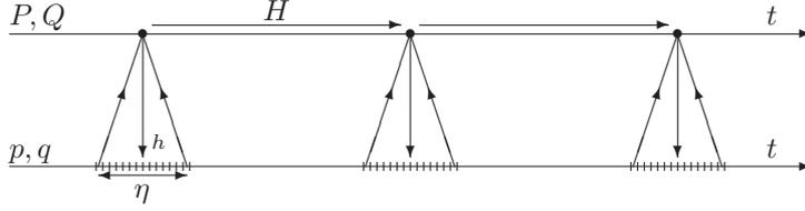
FIG. 2.2. Schematic description of the relation between macro and micro integration: synchronous algorithm
